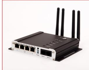
The module deployed, an Eseye Hera 604 with add-on logger functionality, can store all data and publish to AWS as required, ensuring there is no loss of information. A key challenge to the solution is to deliver secure and resilient connectivity, otherwise the farmers' data will be void.
