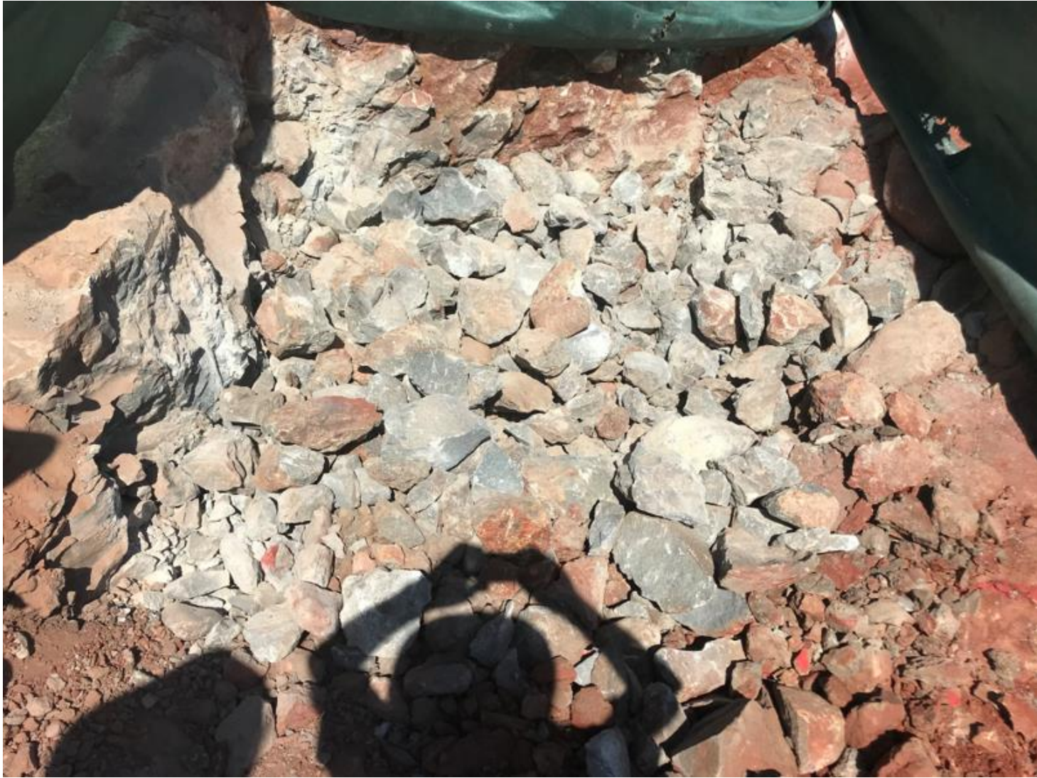
(Figure 3: Sample site at Comet Well. 2 x 2 m pit from which a sample has been chiseled. Rock pieces must be less than 0.2 m across in order to fit in the crusher at SGS Minerals.)
