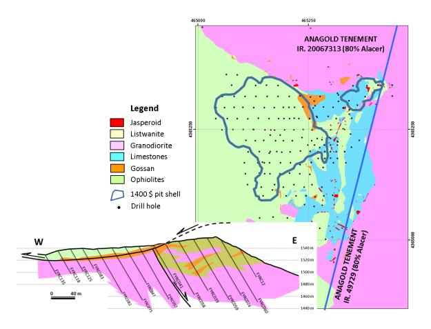
**Çakmaktepe Southeast Resource**: Blue drill hole collars represent drilling previously reported and incorporated into the 2017 Çakmaktepe Mineral Resource estimate. E-W cross section shows Jasperoid and gossan confined (and controlled) to the ophiolitic thrust zone.
