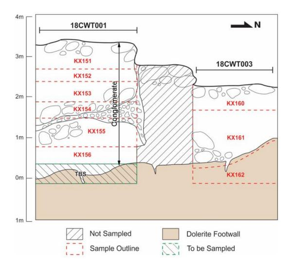
(Figure 2: Illustration showing samples taken from the basal bouldery conglomerate exposed in trenches 18CWT001 and 18CWT003 at the Powerline showing at Comet Well. Dip of the units is to the left. Each bulk sample is collected from a 2 x 2 m subhorizontal panel at least 0.3 m thick. Samples weigh approximately 5 tonnes or greater. Footwall dolerite is also routinely sampled. Novo plans to use bulk samples such as these to assess the grade of the conglomerate package.)
