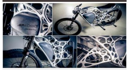
The world's first 3D printed electric bike aluminium-scandium frame makes it lighter and stronger
