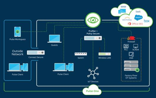
Pulse Policy Secure and Pulse Connect Secure tie contextual user data to network and application access, addressing regulatory compliance and audit demands. Pulse Secure Profiler finds factory floor devices and performs pre-connect security compliance. When deployed with popular next-generation firewalls, Pulse Policy Secure provisions user session information and gives additional perimeter-based security. Pulse Secure Access solutions are managed centrally through Pulse One.
